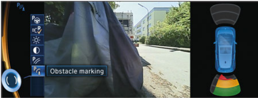
Rear view camera, view in CID, setting obstruction marking
